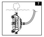
Turn on the filter pump and make sure water is flowing through the micro-screen (6) and the hose adaptor (7). The auto cleaner is now moving and vacuuming the pool floor. See Fig. 8.
