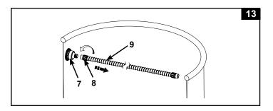
3. Unscrew (counter-clockwise direction) the hose adaptor (7) from the threaded strainer connector. Remove the micro-screen (6) from the hose adaptor. Use a garden hose to clean and flush out any debris from the micro-screen and hose adaptor. See Fig. 14.
