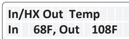
Figure 41. Inlet and Heat Exchanger Outlet Temperature
