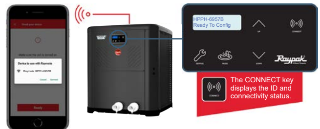
Figure 125. Wi-Fi Access Point Settings
