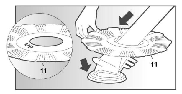
2. Install the Handle by flexing and inserting each end into the slots on top of the cleaner. Install the Deflector in the same manner under the cleaner insuring the weight is towards the bottom.
