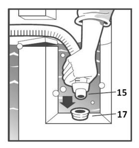
5. If connecting through your dedicated suction outlet, lift the cover and insert the first hose male end directly into the outlet.
