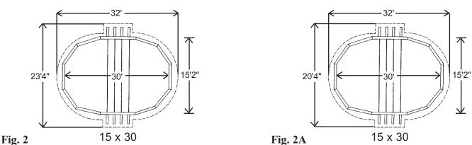
\*Once you have the appropriate area marked out, remove any sod that is in the area. Also be sure to avoid all electrical wires, gas lines, septic tanks, cesspools, dry wells, tree roots, stumps, buried debris, and sudden slopes within 6' of the pool area.
