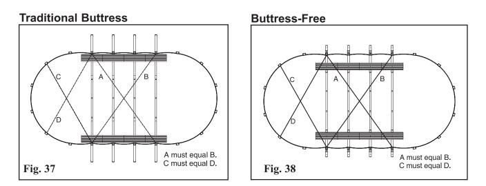
The following are detailed diagrams for every size oval pool that we make. Most of these measurements apply to both the Traditional Buttress oval assemblies and the Buttress-Free oval assemblies. Please use the diagram that applies to your pool to make sure you have everything in its proper position before proceeding with these instructions. Taking a few minutes to check these measurements now can save you major time and efforts down the road if something is not correct.
