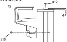
1) Attach the inner top cap using a #12 Screw into hole #2.
