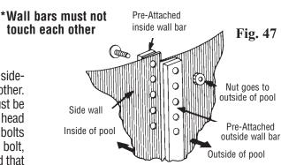
• If you are missing any hardware, do not leave empty holes in the wall joint assembly. Doing so will cause your pool to break! See your pool dealer for additional hardware in the case of a shortage.
