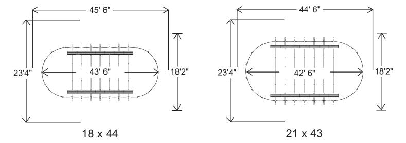
Note: All above diagrams are for Buttress-Free oval pools. If you have a traditional Buttress oval pool, you will need to add 3 feet to the width of the space needed for installation. The length measurement will not change.
