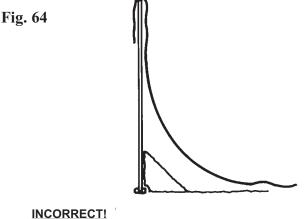
DO NOT LEAVE A GAP BETWEEN LINER AND COVE. THIS WILL CAUSE DOWN-WARD PRESSURE ON THE LINER. CORRECT THIS CONDITION IF IT OCCURS.
