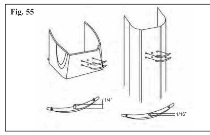
Please note the difference of the accent clips for the resin boot and the steel Upright. For proper fit be sure to use the correct clips.
