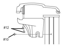
**<u>2 PC RESIN TOP COVER</u>**: Center small half over hole in the top plate as shown and attach with a #12 screw. Slide the large half over the small half and secure using two #10 screws.
