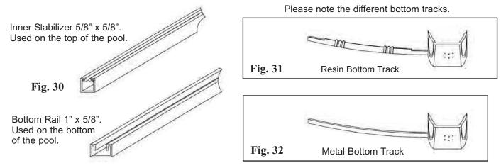
\*IMPORTANT: Make sure you are using the bottom rails and not the inner stabilizer bars. The bottom rails on some pool models are made of resin and not metal (see Fig. 31 and Fig.32). The stabilizer bars are always metal and they have a male and female end. The bottom rails are the larger width rails that have the straight cuts on both ends. The bottom rails do not interlock (see Fig. 30).
