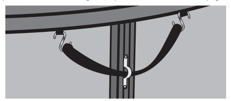
4 Place the felt pad material between the cover's underside and the upright's turnbuckle. (Fig 4)
