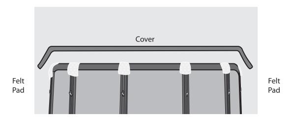
With the cover on and the pad in place attach a bungee cord around every upright. Continue to drill the straps at the set level pre-determined, judgement calls can be made at this point to ensure the cover is not too tight! There should be very little to no tension on the bungee cords at this point.
