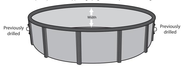
Place cover on top of the pool. Run the supplied bungee cord through the cover's webbing loops and pre-drilled plastic strap (Fig 3). Repeat this step on the other three pre-drilled strap locations. By the end of this step the cover should be snug on the pool and attached to the 4 uprights.
